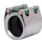
Series 745/01 Repico® grip coupling Universal and tensile for all metal pipes Stainless steel AISI 316 NBR or EPDM sealing DN15-400
