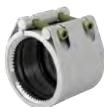
Series 745/01 Repico® grip coupling Universal and tensile for all metal pipes Stainless steel AISI 316 NBR or EPDM sealing DN15-400
