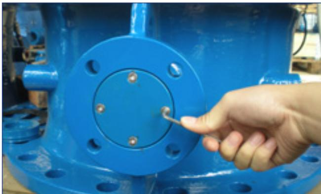
For other bolt dimensions, we recommend application of torques in 4 x thread size, e.g. M12 = 48 Nm.
