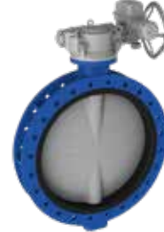
Series 820/20 Centric butterfly valve with loose NBR liner U-section Ductile iron DN150-1600 With any type of actuation
