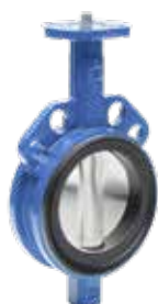
Series 820/00 Centric butterfly valve with loose NBR liner Wafer Ductile iron DN25-1000 With any type of actuation
