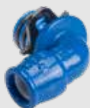
Series 107/31 - 90° push-in fitting for PE pipes Ø32-63 mm, ductile iron. Also available with 45° angle and with Supa Lock™ socket end.
