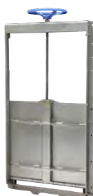
Series 772/63 Penstock, wall-mounted Bi-directional with rising stem Stainless steel AISI 304 200x200 – 1200x1200 mm Options: • non-rising stem • larger sizes, bi-or unidirectional • AISI 316
