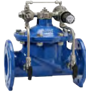
Series 859 Control valve Pressure sustaining DN50-600 PN10/16 Ductile iron/AISI 316
