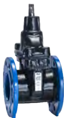
Series 06/52 Premium 100 gate valve Flanged Face-to-face DIN F4 DN40-600 PN10/16 Ductile iron External PUR coating
