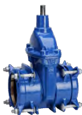
Series 01/70 Supa Plus™ gate valve with tensile coupling ends for PE and uPVC pipes DN40-300 PN16 Ductile iron
