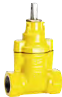
Series 03/25 Service connection valve with internal thread DN25-50 PN4 Ductile iron With external epoxy coating
