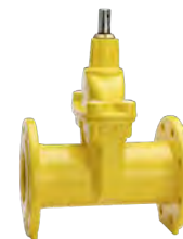
Series 02/70 Flanged gate valve Long DIN F5 DN40-500 PN10/16 Ductile iron With external epoxy coating
