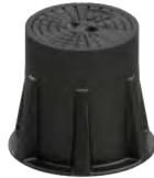
Series 80/39 Surface box for gate valves to DIN 4056 Fixed height Body of PA+ Lid of cast iron
