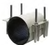
Series 748/02 Repair clamp Single band with support plate Stainless steel AISI 304 or AISI 316 NBR rubber
