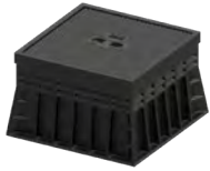
Series 80/37 Surface box for gate valves to DIN 3584 Fixed height Body of HDPE Lid of cast iron
