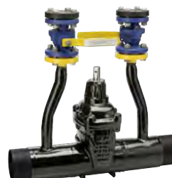
Series 46/80 Gate valve with long spigot ends and two purge points DN80-600 PN16 GP240GH With external PUR coating
