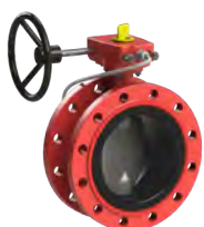
Series 75 Butterfly valve Centric with fixed liner Double flanged short DN50-400 PN10/16 Ductile iron FM approved
