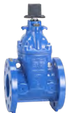
Series 45/59 Flanged gate valve with wrench nut DN50-300 17.2 bar (250 PSI) PN10/16 Ductile iron UL/ULC listed, FM approved
