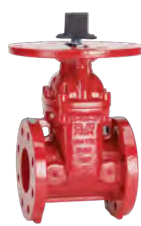
Series 45/5D Flanged gate valve with post indicator flange Alu-bronze stem DN50-400 17.2 bar (250 PSI) PN10/16 Ductile iron UL/ULC listed, FM approved
