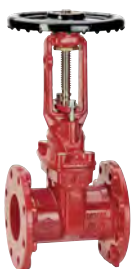
Series 145/46 Flanged gate valve with rising stem OS&Y DN65-200 17.2 bar (250 PSI) ANSI class 150 Ductile iron UL/ULC listed, FM approved
