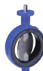
Series 75 Butterfly valve Centric with fixed liner Wafer DN40-1000 Ductile iron With any type of actuation
