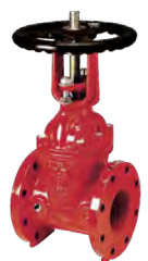
Series 45/56 Flanged gate valve with rising stem OS&Y DN50-300 17.2 bar (250 PSI) PN16 Ductile iron UL/ULC listed, FM approved
