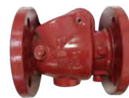
Series 5190/00 Flanged swing check valve Spring loaded Grooved ends to AWWA C606 DN50-200 24.1 bar (350 PSI) Ductile iron UL/ULC listed
