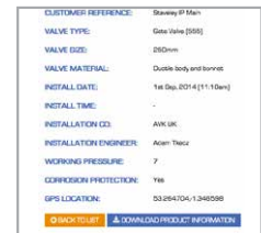
Data record includes: valve type, materials, size, pressure and installer
